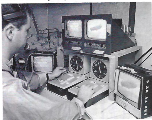
INSTANT REPLAY: Television engineer in ABC control center at football game operates control panels for Ampex HS-100 recorder that provides viewers with an "instant replay" of exciting game action. Time counters (center of picture) indicate when play began so operator can return to that point to replay a segment of action. Television screens show what is picked up by television cameras and what is being aired. Lever in engineer's left hand allows him to control the speed of an "instant replay" so viewers can watch exciting maneuvers in slow motion. HS-100 systems are in use at television stations and networks throughout the world.
