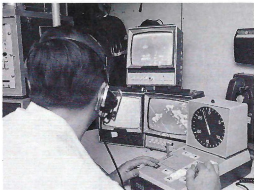
SUPERIMPOSED SCORE: While ABC engineer prepares to show an "instant replay" of a segment of exciting football action during a recent college game, the network superimposes the score of another game over the picture of the playing field. Modern television equipment, such as the "instant replay" recorder and TV switchers which permit special video effects, enable television stations and networks to keep the viewers' interest even during a lull in the game being covered.
